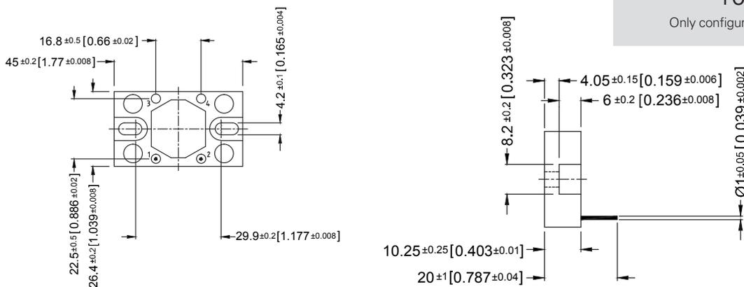
Boreholes distance from min. 30.0 mm to max. 37.0 mm
