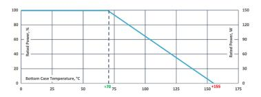
Derating (thermal resist.) AXP-150: 1.76 W/K (0.57 K/W)
