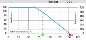
Derating (thermal resist.) UXP®-600: 8.33 W/K (0.12 K/W) Power rating: 600 W at 85°C bottom case temperature\*
